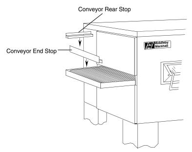
Figure 2-14. Installing Rear and End Stops
